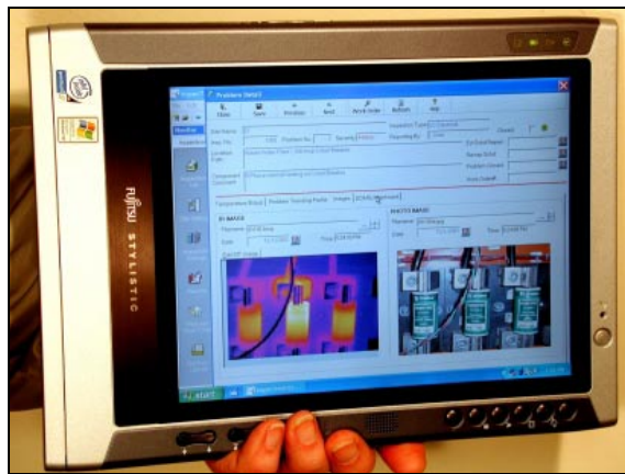
Portable Pen Computer running the InspeCTrend PdM Inspection Management Software
